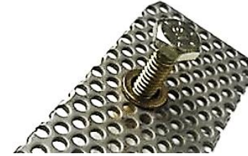
Factory Safety Bolts and Nuts are Used to Mount One Side of the Box to a Roof Rib of the Bus Ceiling
